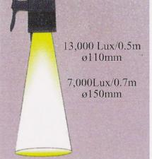
The lamp head consists of a double-wall construction with a heat absorption glass, an inner aluminum isolator, and a heat resistant plastic lamp housing with highly effective ventilation holes; therefore, this design minimizes heat emission and maximizes cold light illumination.
